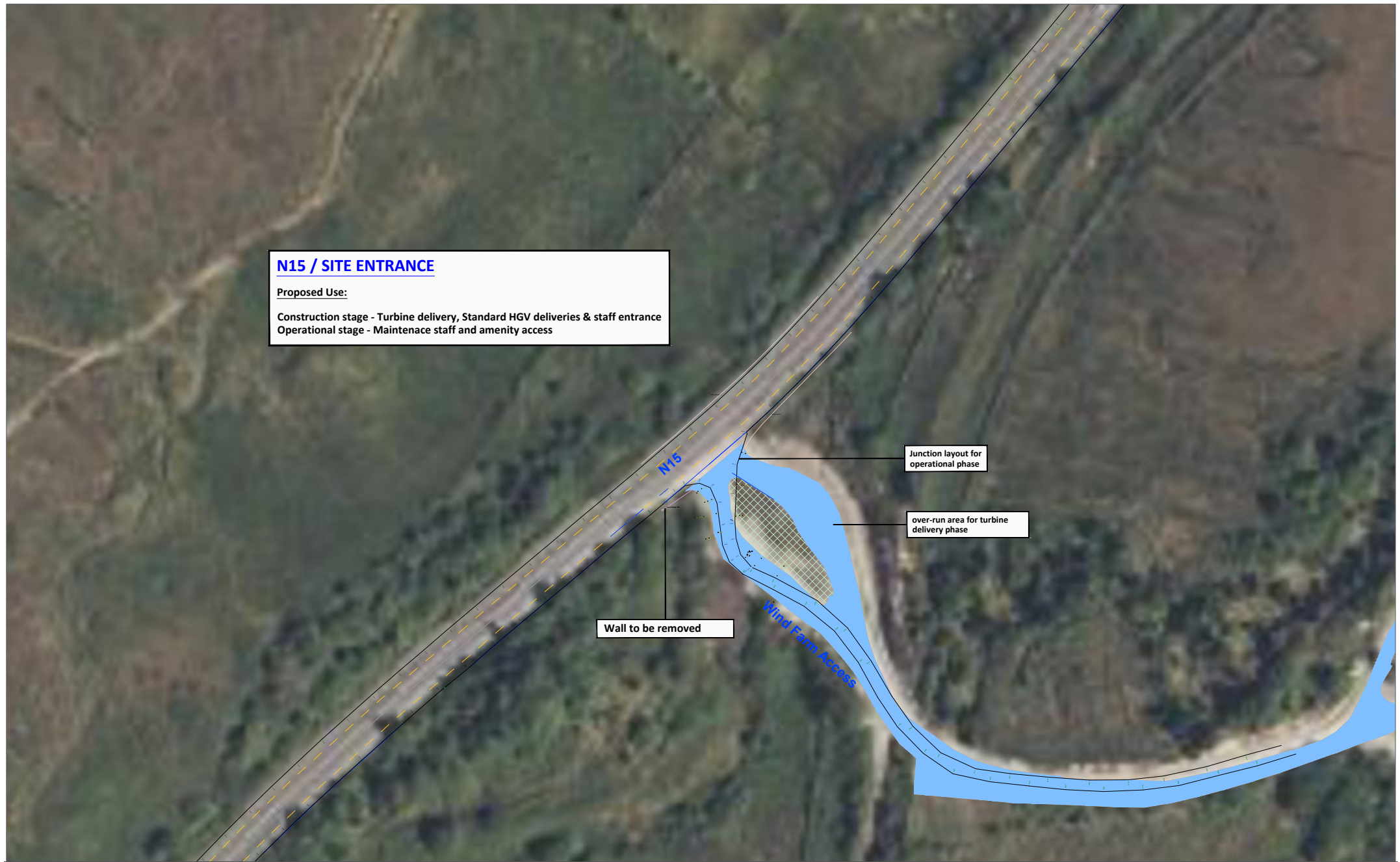
Figure 15-14 Location 10 - Access junction on N15, junction layout
